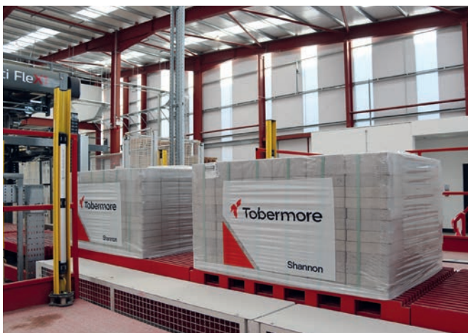
Paver packs strapped, stretch hooded, printed with Tobermore logo, ready for transportation
