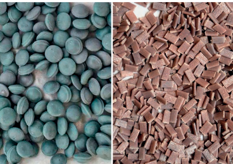
Only a small selection of the granules available. Lentil shape or flakes from recycled plastics
