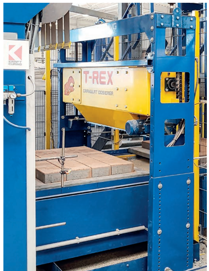
Light barriers detect the products and start the dosing process
