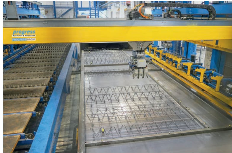
The Wire Center installs transverse reinforcement with and without spacers as well as longitudinal reinforcement and lattice girders according to CAD specifications.
