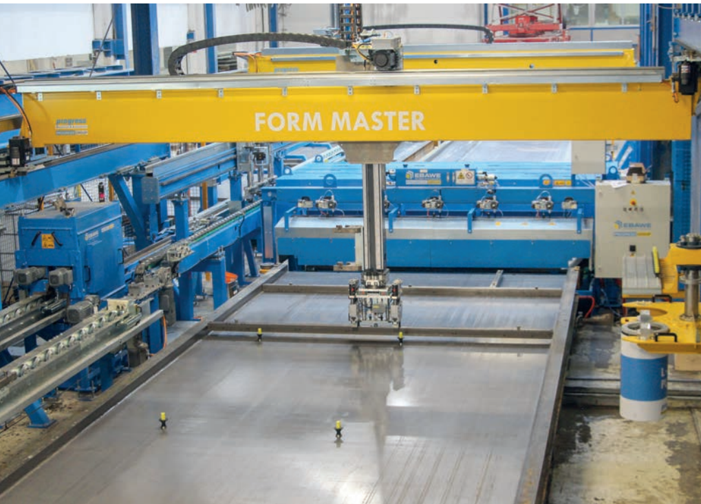
The individualised shuttering robot at Schwörer places the shuttering, magnets and assembly sleeves precisely on the pallet.
