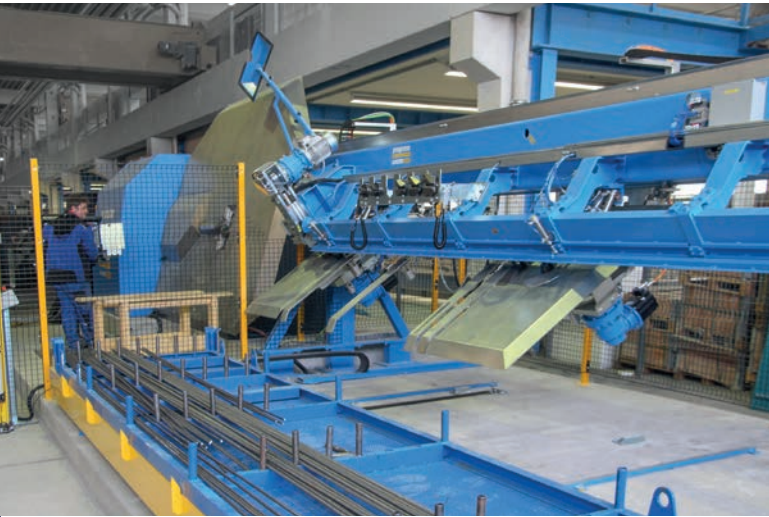
In operation at Schwörer Bausysteme GmbH since the beginning of 2021: the Pluristar - a multifunctional machine for all steps in steel processing from the coil.
