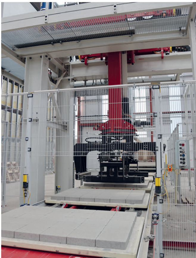
One of three Hess cubers Servo 900 belonging to the new circulation system in production hall IV at the Tobermore site
