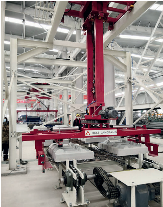
Figure 6: Automated sleepers stacking device
