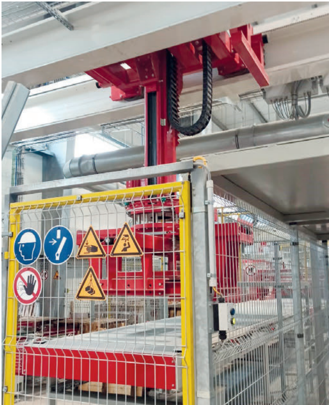
Layer stacker with carriage and motorised 4-sided clamp
