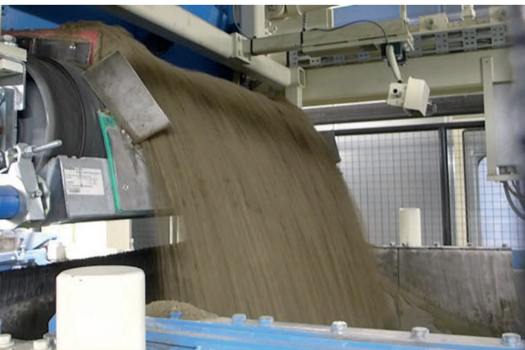
Filling box feeding via dosing belt.
