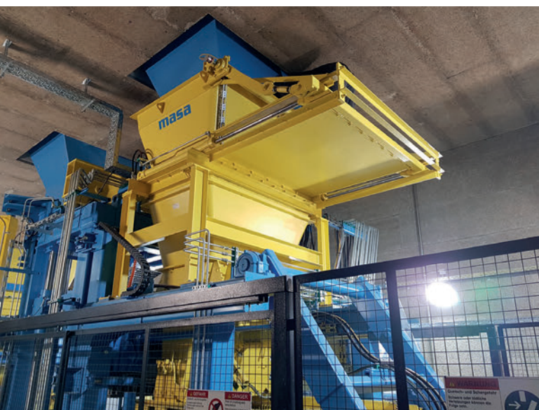
Hydraulic version for the block making machines of the XL series
