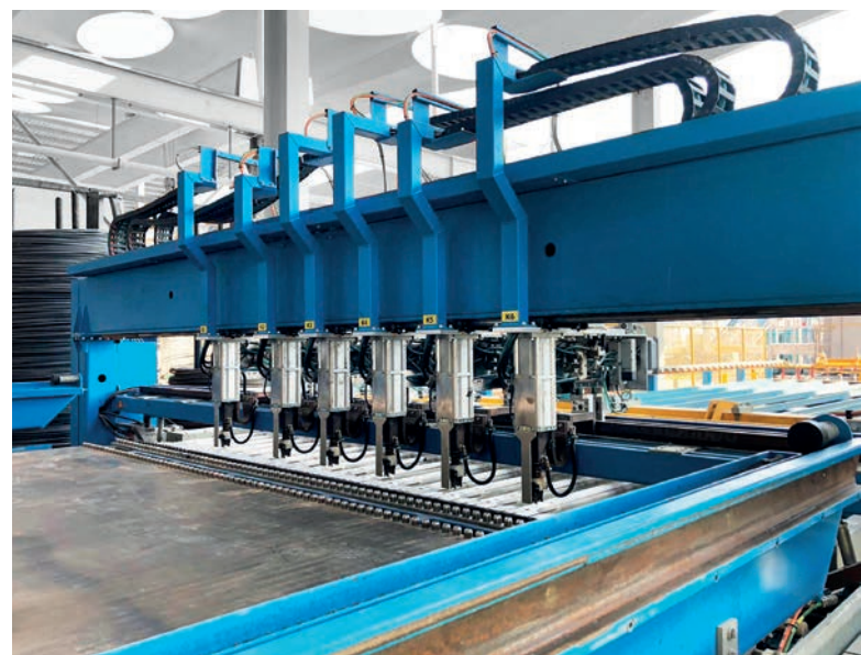
Reinforcement meshes are produced on the M-System BlueMesh® mesh welding machine with an exact fit and just-in-time.
