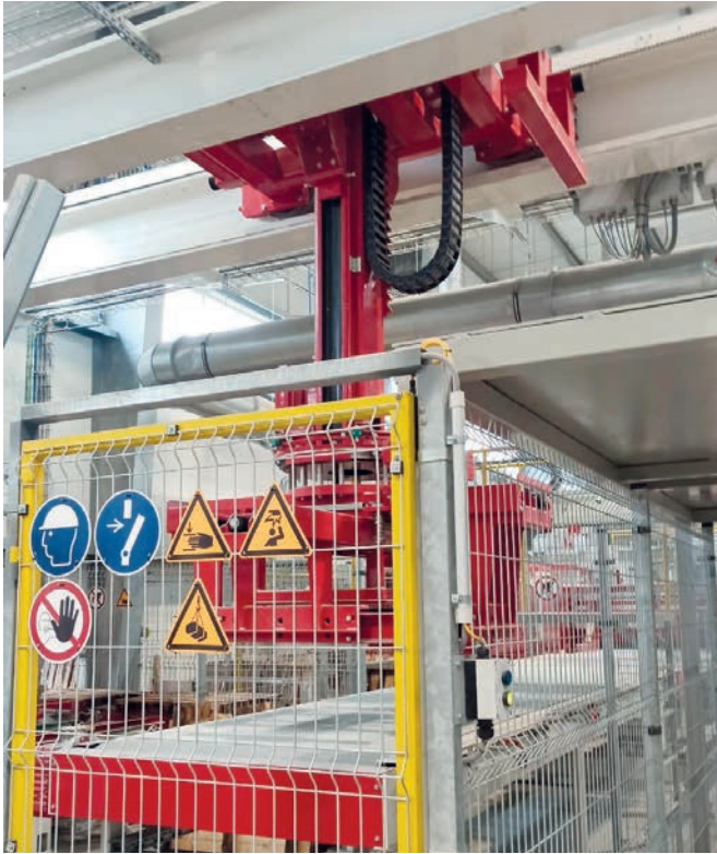
Layer stacker with carriage and motorised 4-sided clamp
