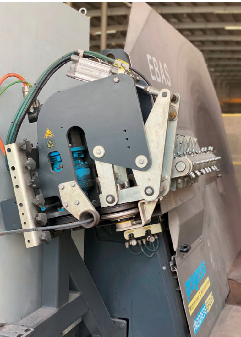
The EBA S 16 automatic stirrup bending machine from Progress Maschinen & Automation is successfully used for processing reinforcing steel.
