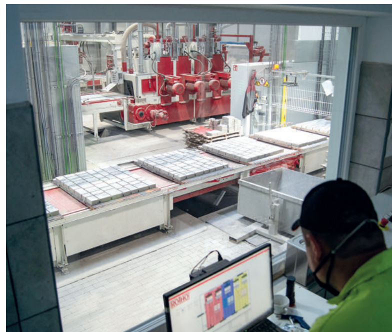
View from the control cabin towards the dry side; in the background is the SR Schindler curling machine
