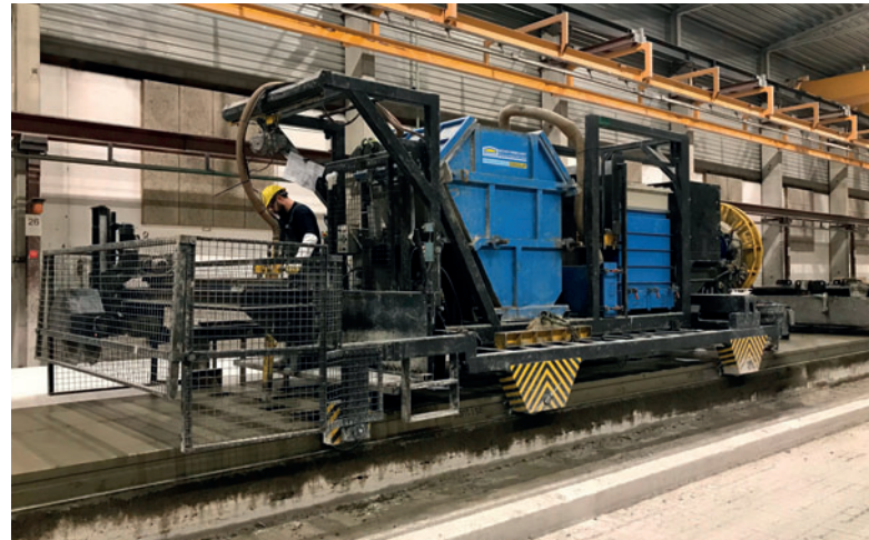
The Concrete Aspirator is equipped with a suction nozzle and associated pump that conveys the extracted fresh concrete through a hose into a waste container. The additional double cut saw module is visible at the front of the machine.
