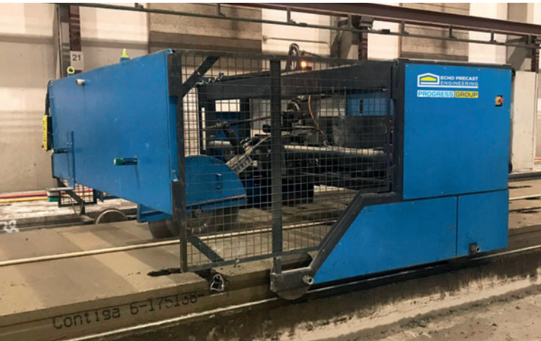
The Fresh Concrete Saw FCS makes longitudinal cuts on fresh concrete.
