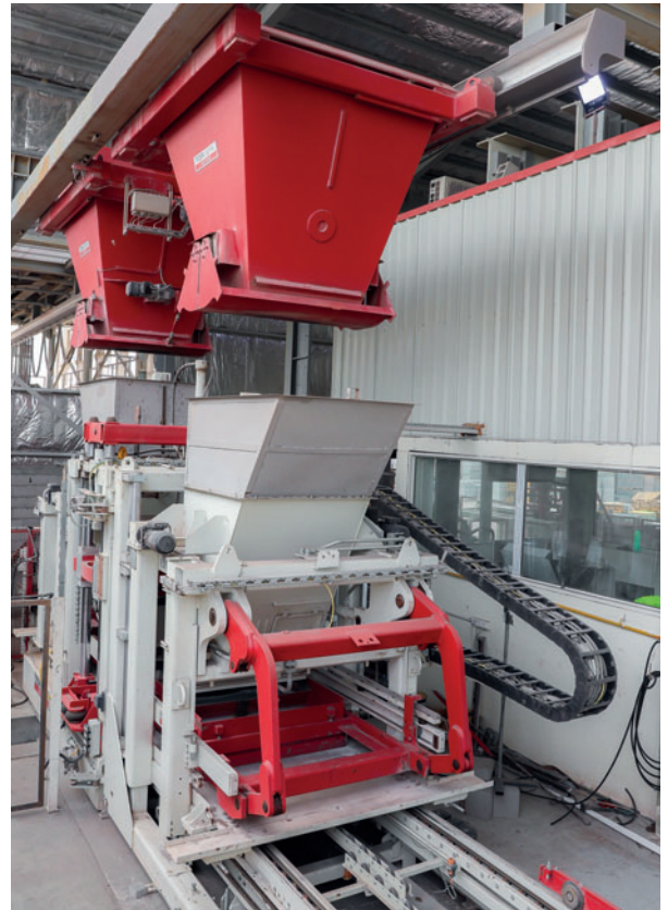
Block machine RH 1500-3 with double flying bucket
