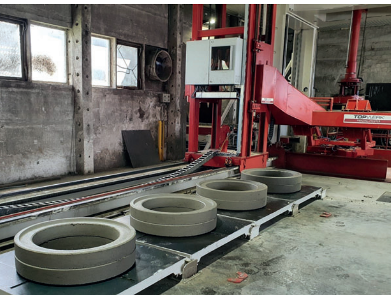
With the universal insertion robot for base pallets, the compensation rings are placed on boards from the production area next to the machine
