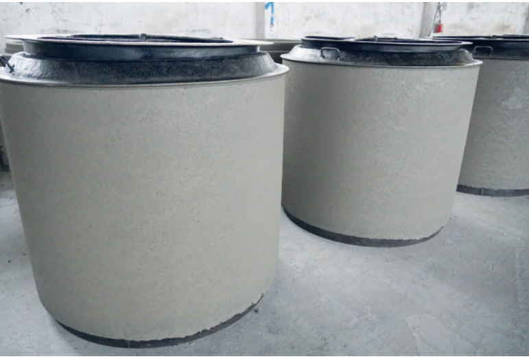
Freshly produced manhole rings in the curing area
