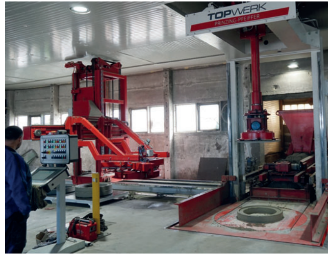
Tornado, production of compensation rings
