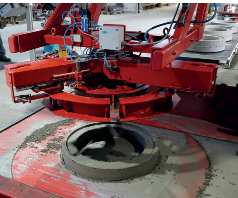
Attached gripper for transporting the compensation rings
