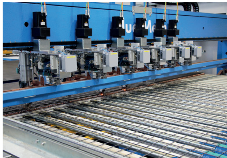
Individual steel wires can be welded at any distance desired using the Progress spot welding process
