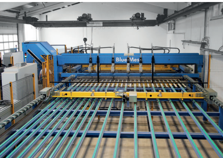
The new M-System BlueMesh® mesh welding system makes it possible to produce made-to-measure reinforcing meshes flexibly
