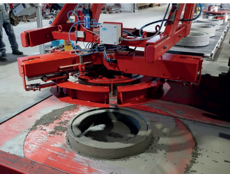
Attached gripper for transporting the compensation rings
