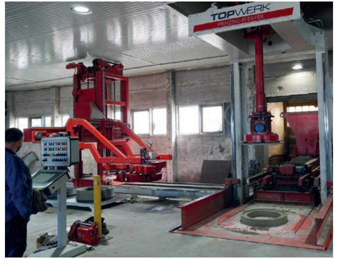
Tornado, production of compensation rings
