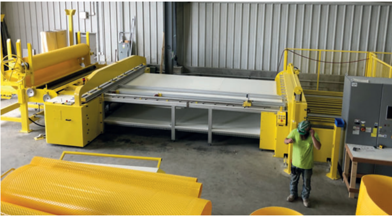
The fully automatic HDPE liner welding system from Schlüsselbauer Technology supplies liner cylinders from DN 300 to DN 1500 for a max. pipe length of 3 m.
