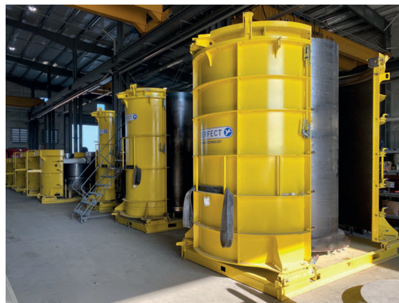
The Perfect Forming Technology moulding system for processing self-compacting concrete is a key element of the Perfect Pipe production process.
