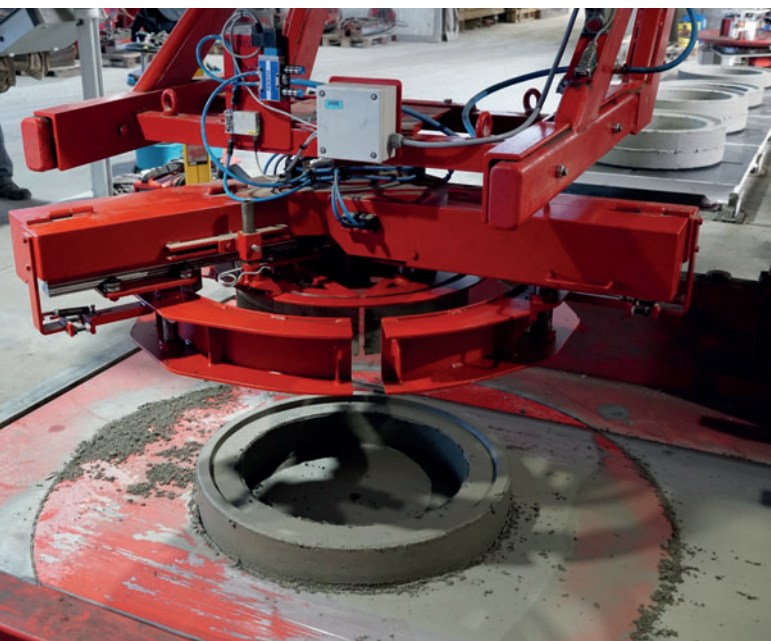
Attached gripper for transporting the compensation rings
