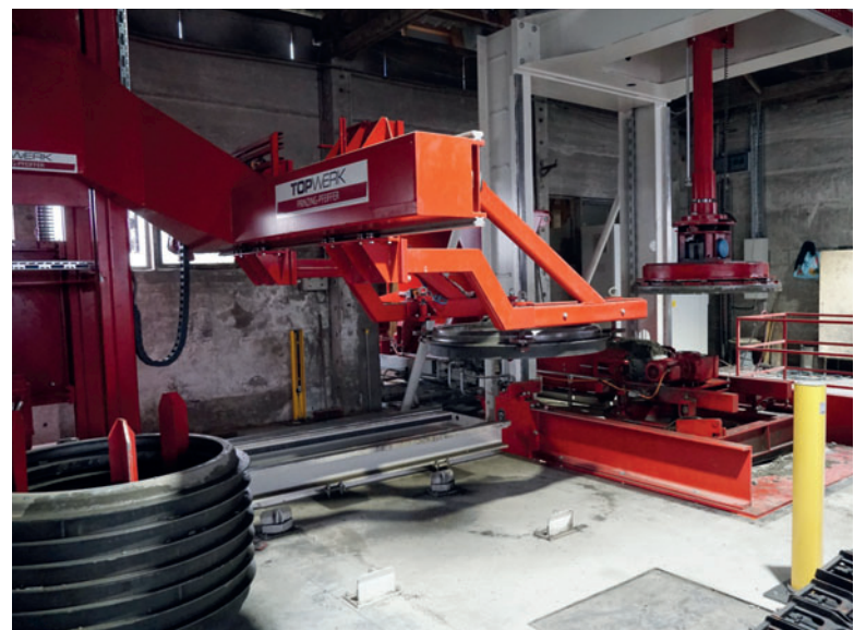
The base pallet insertion robot with stacked base pallets
