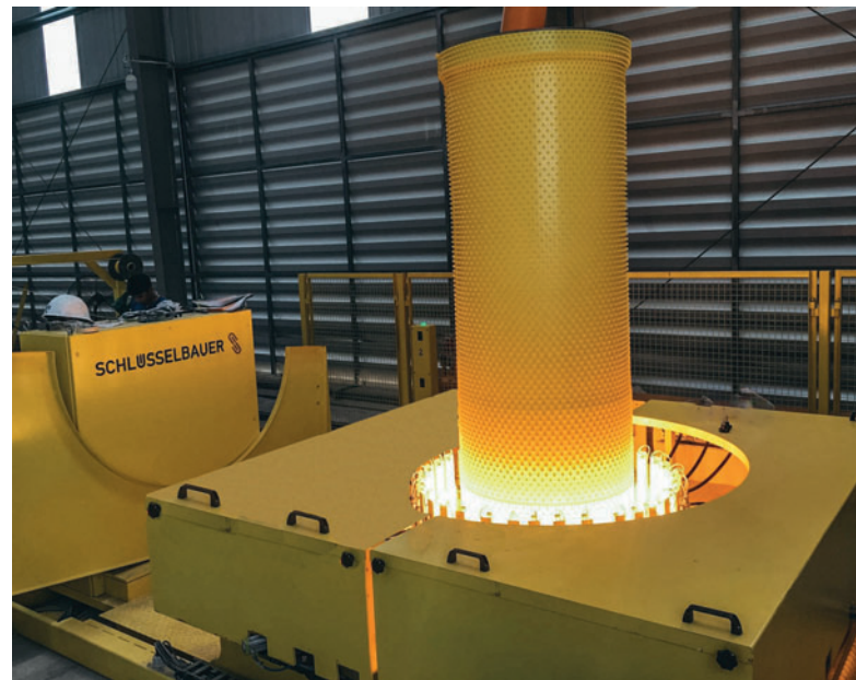
The thermoplastic forming of the liner cylinders is an essential step in the production of Perfect Pipe
