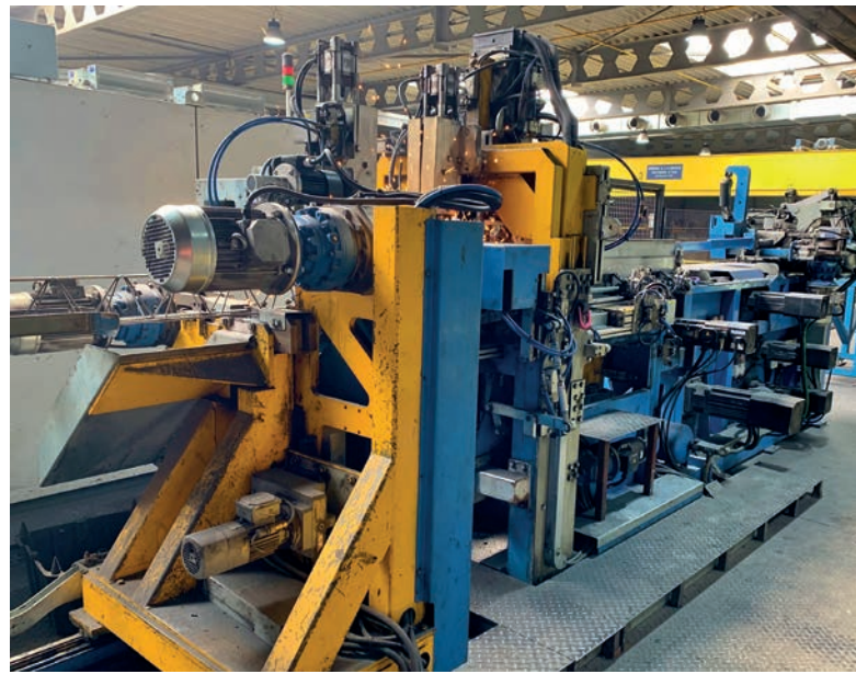
The VGA Versa lattice girder welding machine produces just-in-time lattice girders in different heights for the carousel plant and is equipped with an automatic top wire diameter change.
