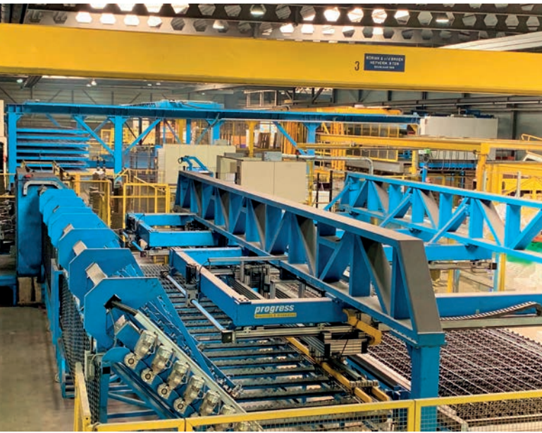
The M-System mesh welding plant was developed for the most flexible production possible and thus fits very well into the overall concept.
