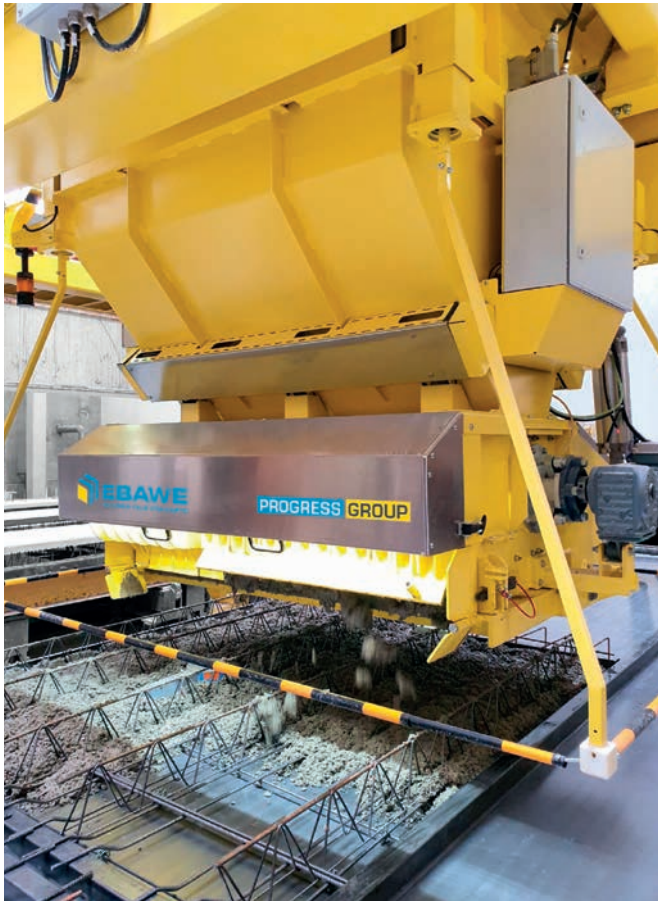
The new concrete spreader works quickly and precisely in the production of double walls with and without insulation, precast slabs with in-situ topping and solid walls in very high quality.
