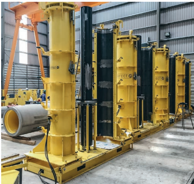
User-friendly molds of the category Perfect Forming Technology from Schlüsselbauer in production at Phnom Penh Precast Plants, Cambodia
