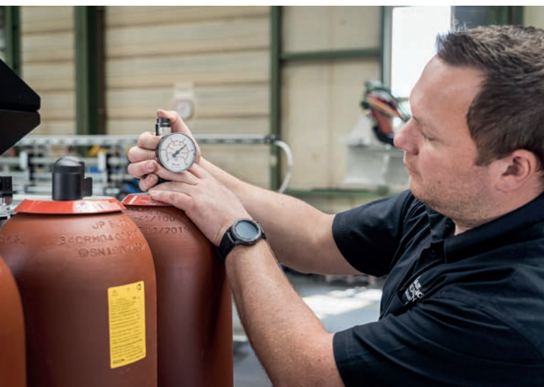
Testing of the bladder accumulator for constant performance and safe operation
