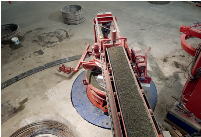
The Prinzing Pfeiffer Variant is an individually adaptable machine concept for the production of concrete or reinforced concrete pipes (round and non-circular, with or without base), inliner pipes, jacking pipes, box culverts, etc.
