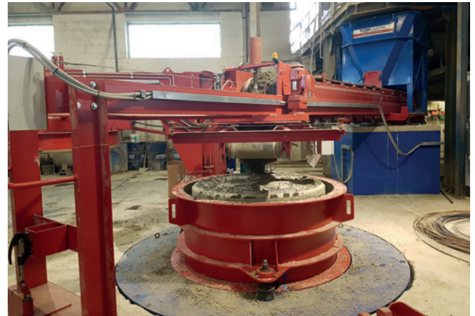
The Prinzing Pfeiffer Variant is an individually adaptable machine concept for the production of concrete or reinforced concrete pipes (round and non-circular, with or without base), inliner pipes, jacking pipes, box culverts, etc.
