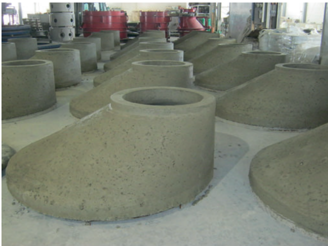
The new manhole ring and cone production on the Variant 2000 C was configured according to the same principle as the existing machine: medium quantities with nominal widths up to 2,000 mm and removal of the products in the mould jacket to the curing station.
