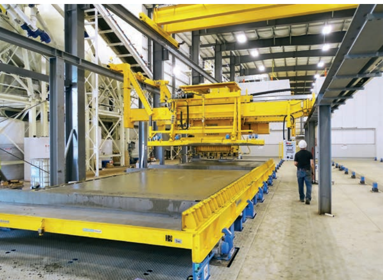
Huffcutt Concrete Inc. manufactures solid wall elements in the new plant and can offer them with an extremely short delivery time.
