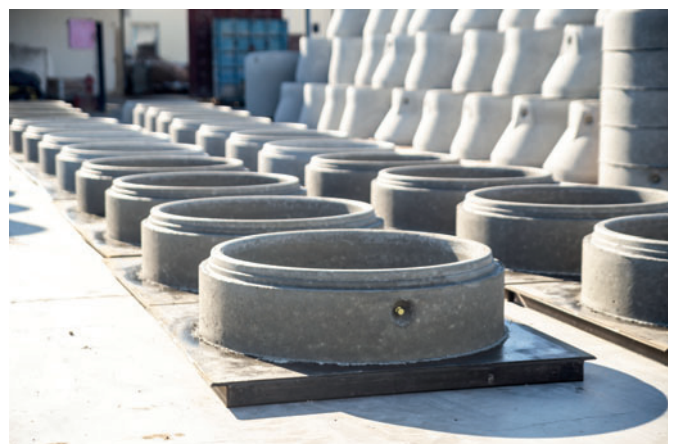
Ball head anchors, securely compacted into the concrete using vibration, provide the basis for safe handling through to its installation on the construction site. © Vojtěch Peša
