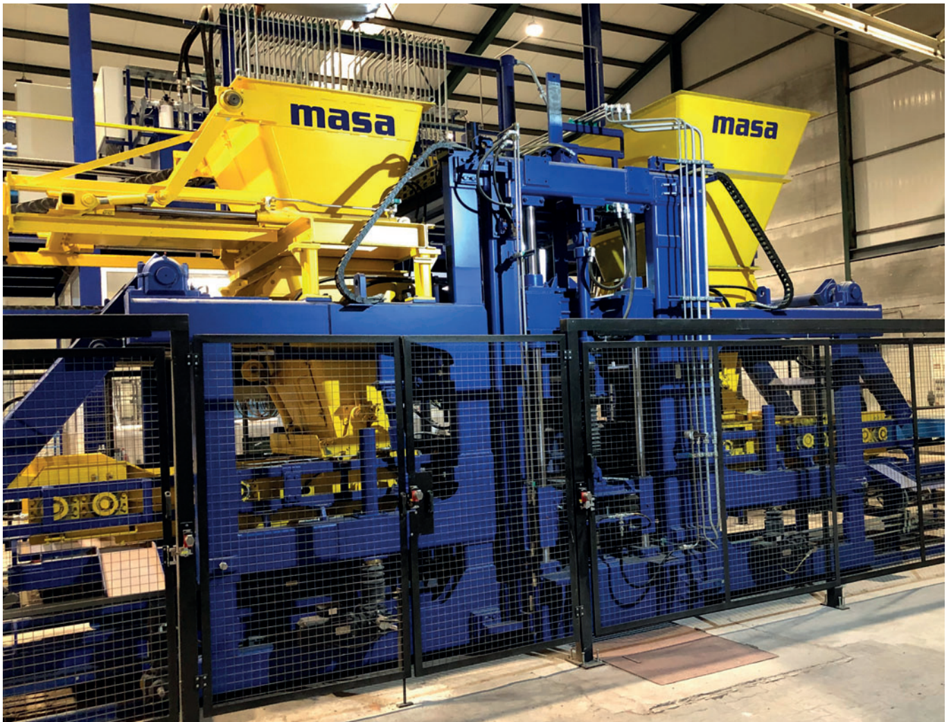
Masa block making machine L 9.1 for the production of concrete blocks with or without face mix layer
