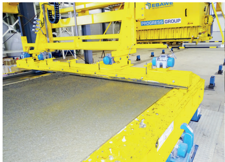
The levelling beam attached to the concrete spreader draws off the concrete and compacts it according to the depth of the concrete layer.
