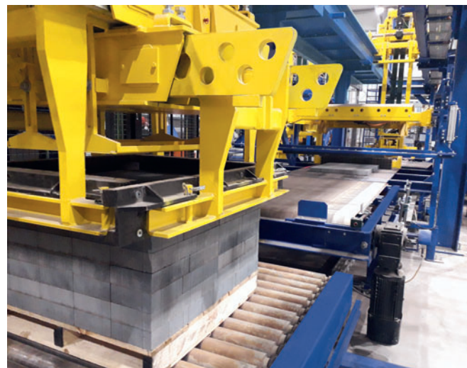
Cubing of the finished products
