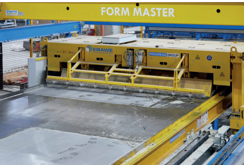
In the new circulation plant at HTB Hoch- und Tiefbaustoffe GmbH & Co KG in Könnern, the pallet surface is optimally cleaned by the pallet cleaner after deshuttering.
