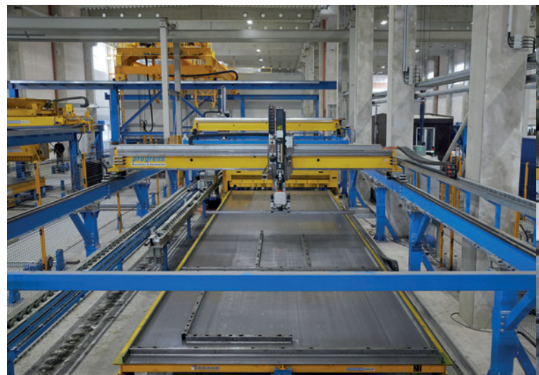
The combined shuttering and deshuttering robot from progress Maschinen & Automation works with the Infinity Line® shuttering system, which significantly reduces the amount of shuttering required and enables very high-quality outer edges to be produced.
