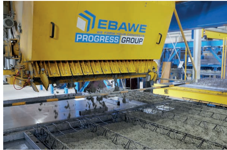
The new concrete distributor from Ebawe takes over the fully automatic concreting of the precast slabs with in-situ topping and double wall elements.
