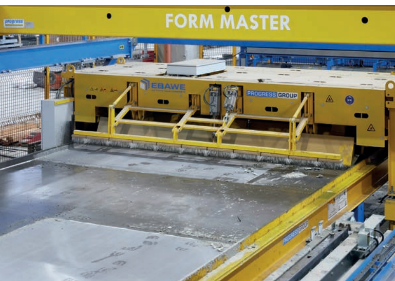
In the new circulation plant at HTB Hoch- und Tiefbaustoffe GmbH & Co KG in Könnern, the pallet surface is optimally cleaned by the pallet cleaner after deshuttering.
