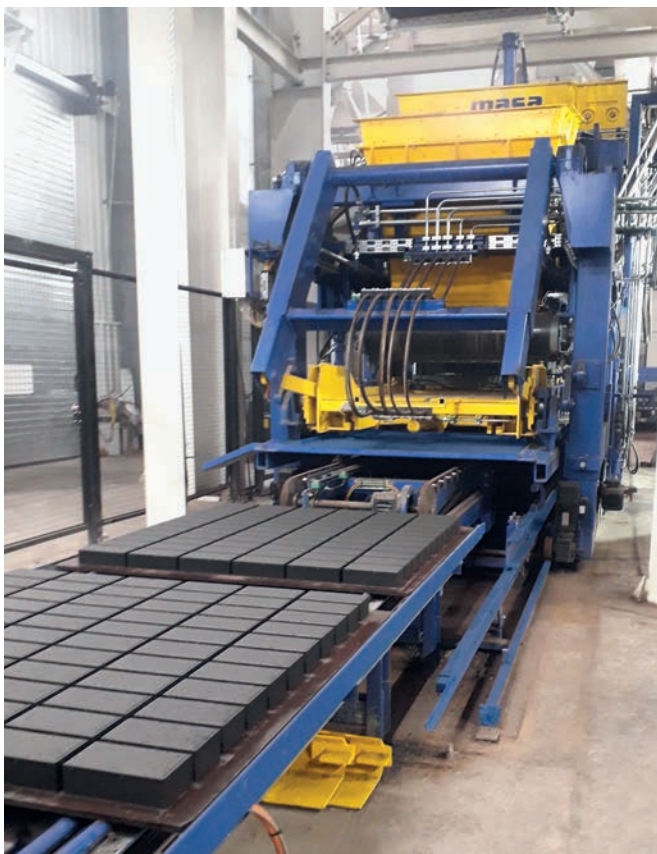
Masa block making machine XL 9.2
