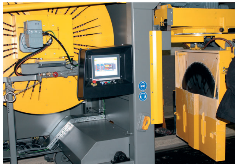
The multi-angle sawing machine has both an Internet connection and an external operator touchpad (Photo: Dennert).
