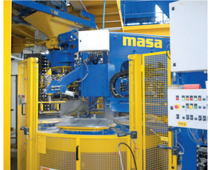
Face mix distributor, back mix concrete feeding, mould changing station, in conjunction with a safety concept with lowerable safety grids.
