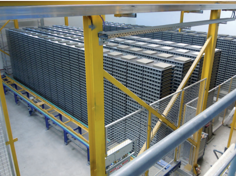
Pallet storage grab for maximum utilisation of the storage area (before and after the later housing and installation of the curing system).
