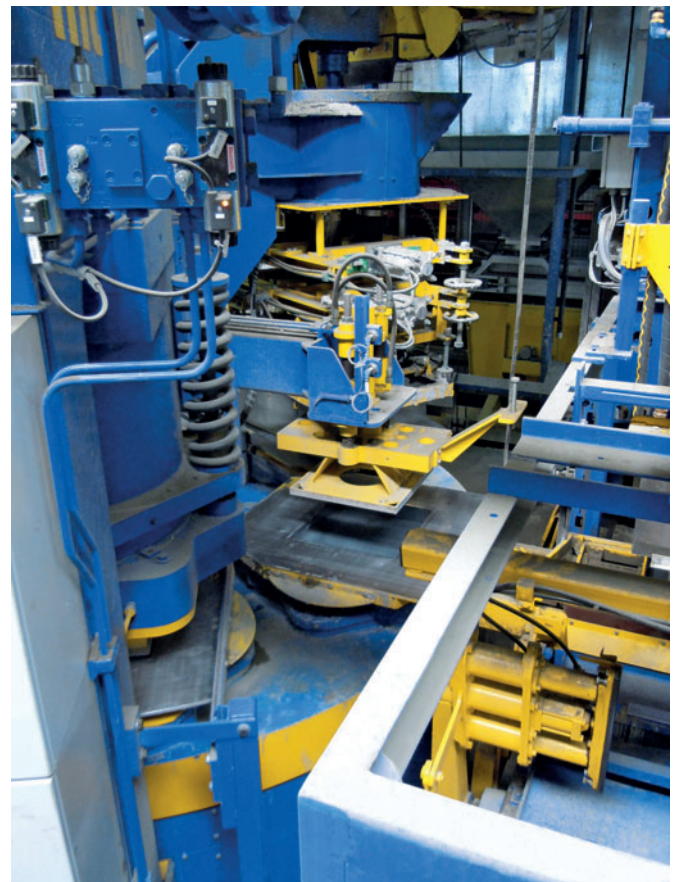
Ejection station with removal device (with a hose type batcher in the background)
