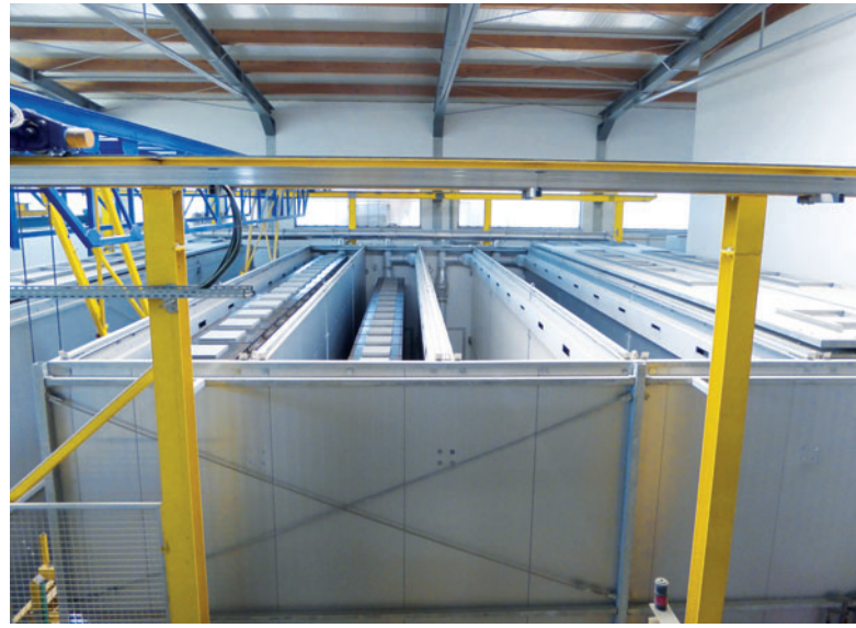
Pallet storage grab for maximum utilisation of the storage area (before and after the later housing and installation of the curing system).
