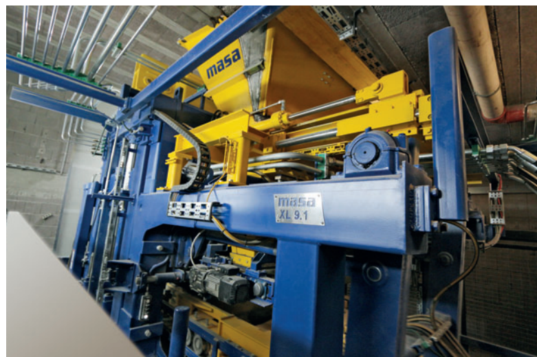
Integrated in the concrete silo: The proven Masa multi-colour device.
