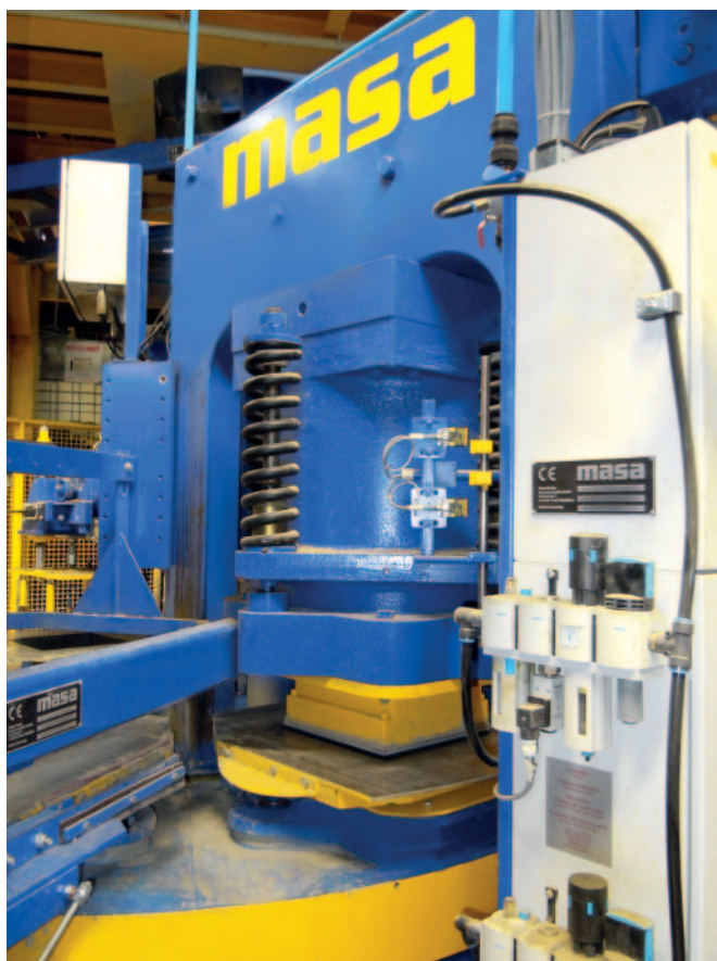
Station de compression principale
