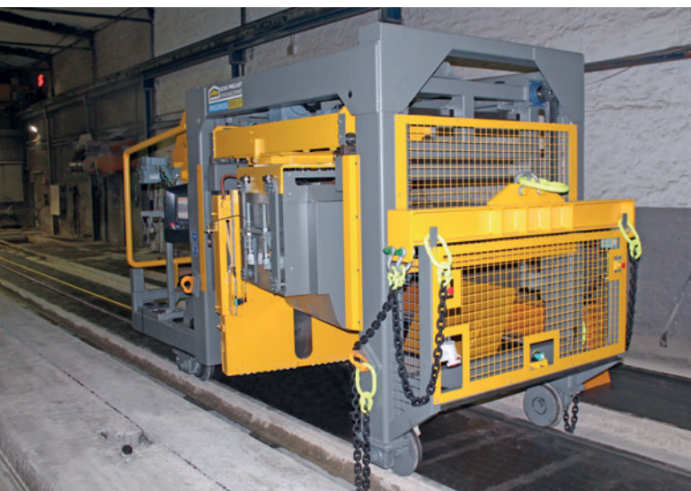
The MAS 1100 from Echo Precast provides Dennert with a higher degree of automation and a more efficient production of prestressed hollow-core slabs (Photo: Dennert).
