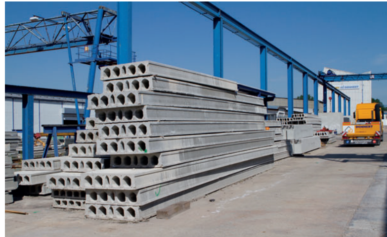
Since the 1970s, Dennert has been manufacturing prestressed hollow-core slabs in the Upper Franconian key field for versatile use (Photo: Dennert).
