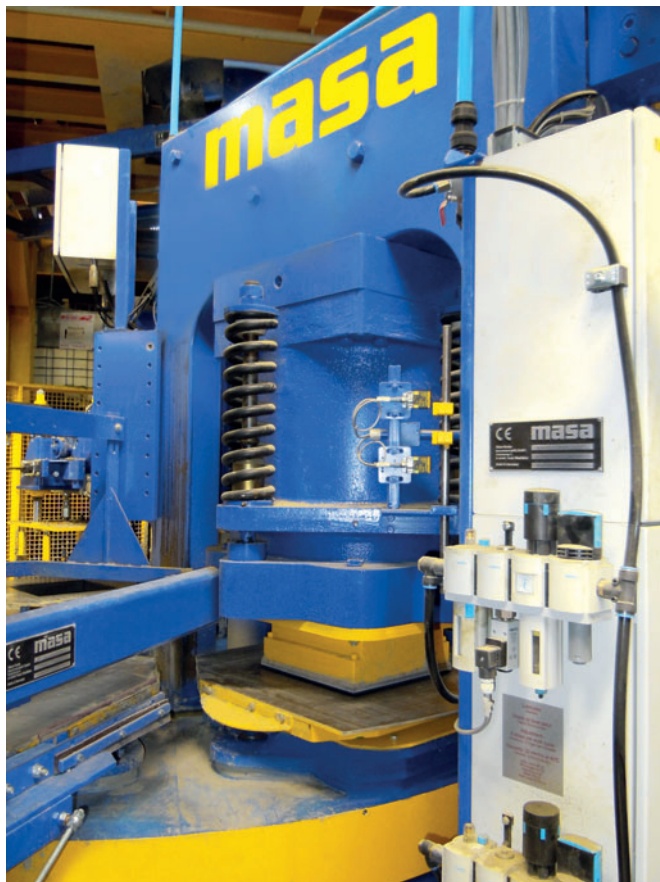
Main pressing station
