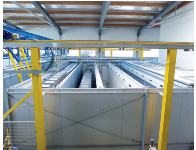
Pallet storage grab for maximum utilisation of the storage area (before and after the later housing and installation of the curing system).
