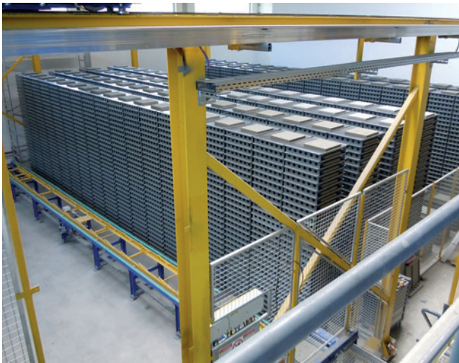
Pallet storage grab for maximum utilisation of the storage area (before and after the later housing and installation of the curing system).
