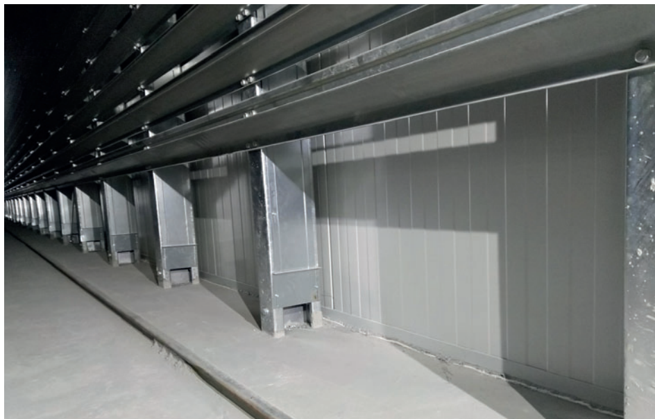
Fig. 5: Every single perimeter column of the Kraft rack functions as an air duct, heating the chamber floor, thus avoiding condensation and eliminating corrosion. (Picture: Kraft Curing Systems)
