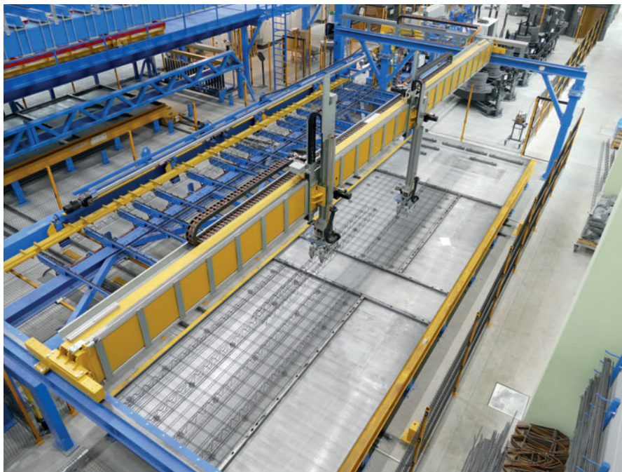
A multi-axis linear robot rounds off the automated reinforcement area in Eder's new plant.
