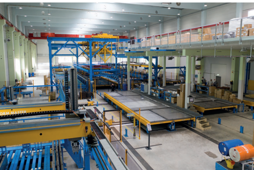
View of the new, highly automated circulation system at Systembau Eder in Kallham
