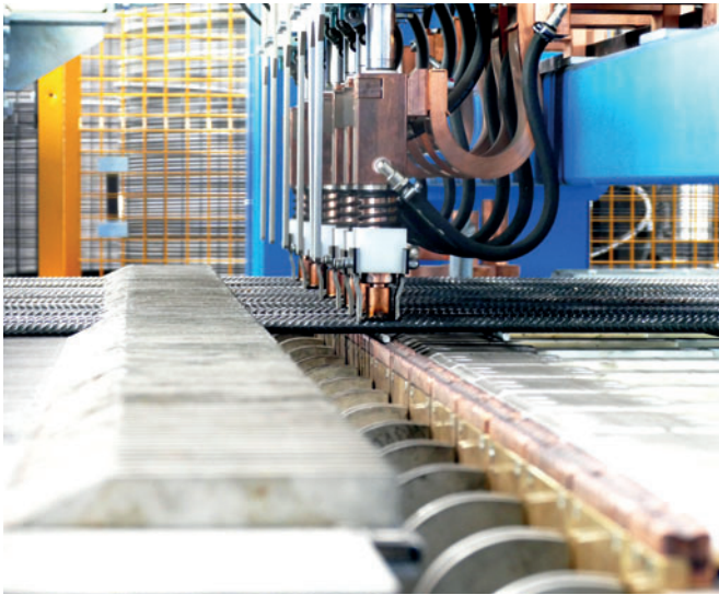
Just-in-time production of reinforcement meshes with the BlueMesh mesh welding machine from progress Maschinen & Automation
