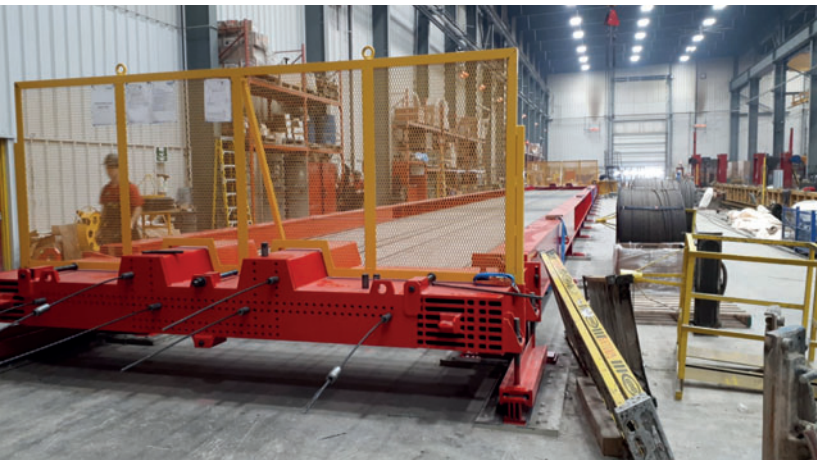
2.7m x 34m self-stressing universal casting bed with 560 tons of prestressing capacity
