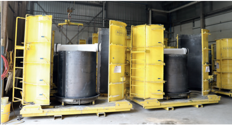
The moulds have a two-piece mould shell and can be pulled apart symmetrically.
