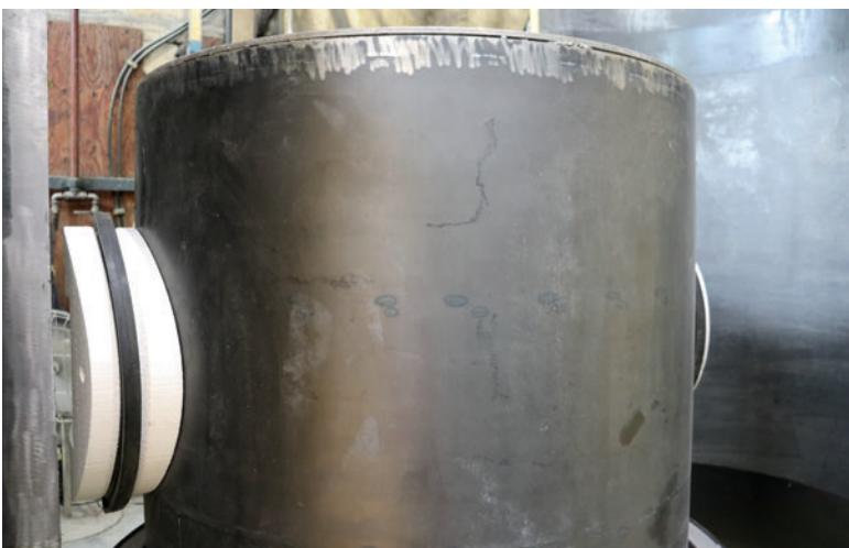
The negative bodies for pipe connections with integrated gasket can also be applied directly onto the steel core of the mould.
