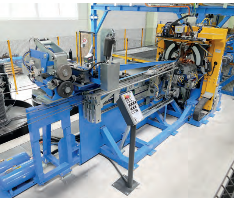
With the highly flexible VGA Versa lattice girder welding machine, the lattice girders are produced "just in time", which enables Eder to achieve high savings potential in logistics, storage costs and waste.
