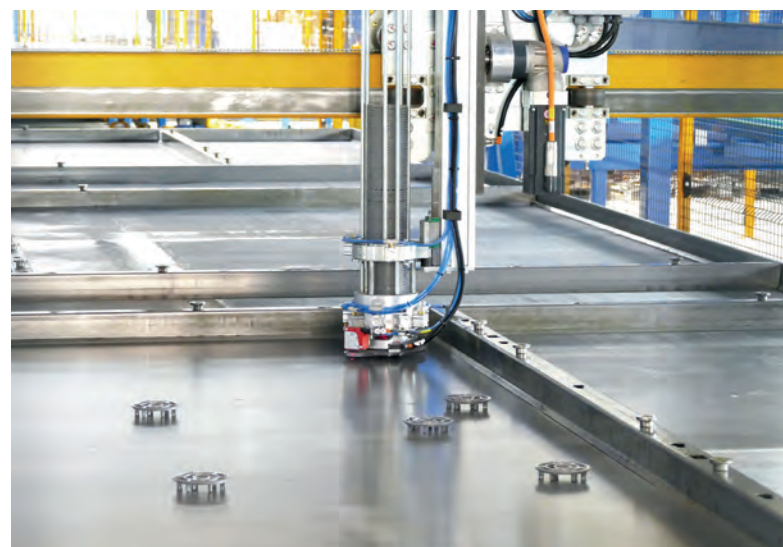
Eder achieves high savings through the fully automatic setting of spacers with the MeshSpacer.
