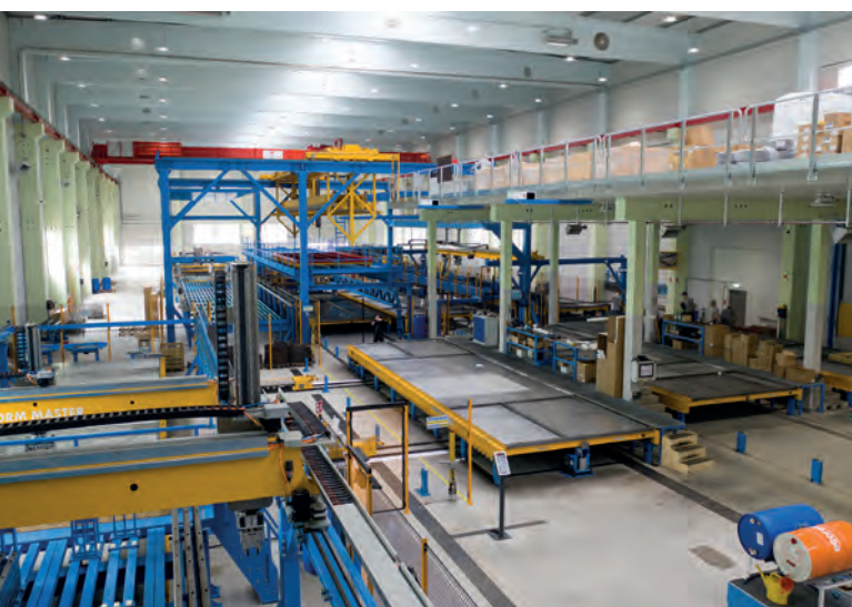
View of the new, highly automated circulation system at Systembau Eder in Kallham
