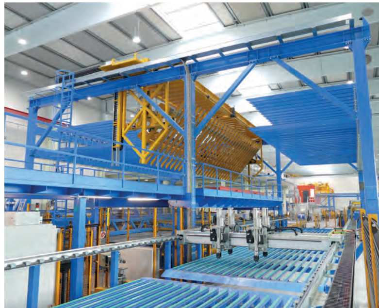
The magnetic crossbeam inserts the meshes into the pallets according to CAD specifications, serves the intermediate buffer, can turn the meshes when longitudinal bars have to be above the cross bars and places the meshes on a stacking carriage.
