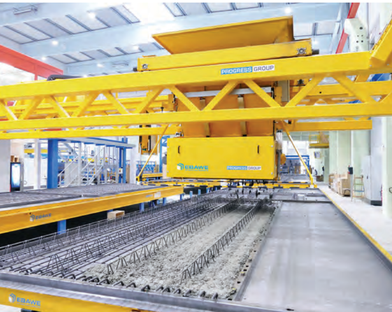
High discharge speed paired with very good concrete dosing capability thanks to the new eCon® Drive automatic concrete distributor
