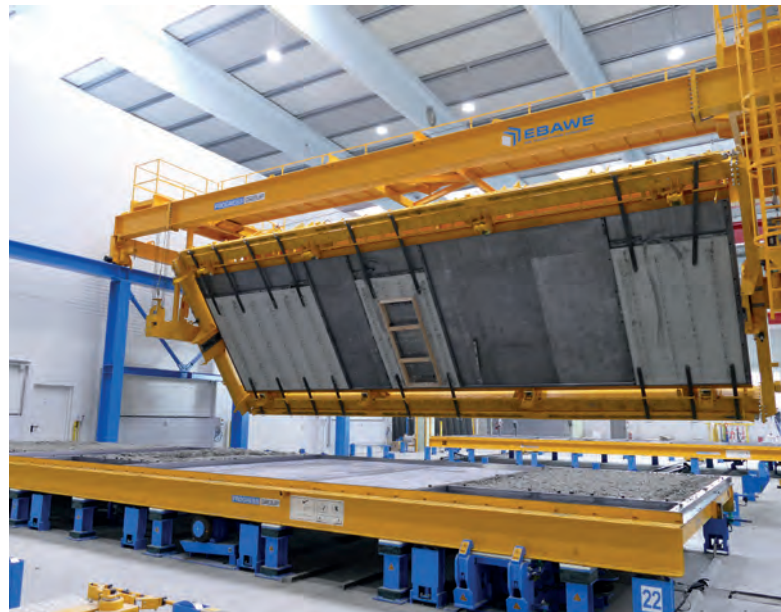
In addition to precast slabs with in-situ topping, Eder also manufactures double walls with and without insulation - the ergonomic turning unit takes care of the turning process.
