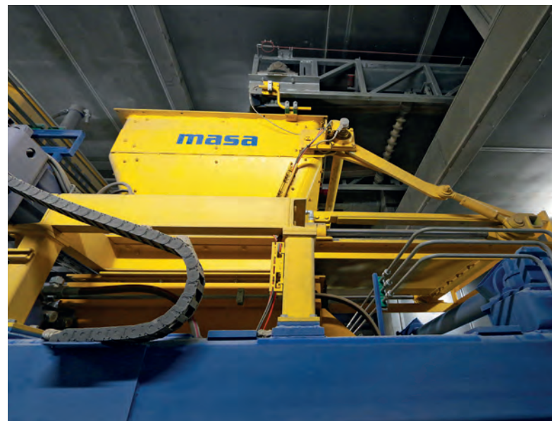
Multi-color device with hydraulically driven slider
