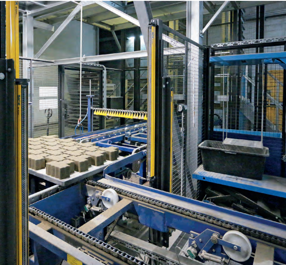
Modular V-belt conveyor system with quality control station
