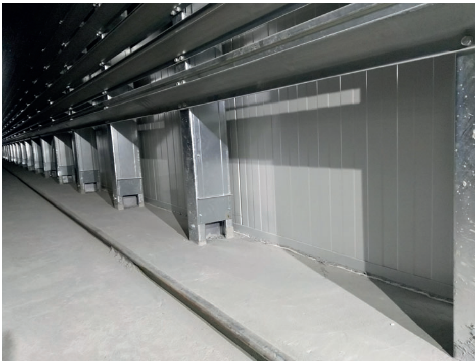
Fig. 5: Every single perimeter column of the Kraft rack functions as an air duct, heating the chamber floor, thus avoiding condensation and eliminating corrosion. (Picture: Kraft Curing Systems)
