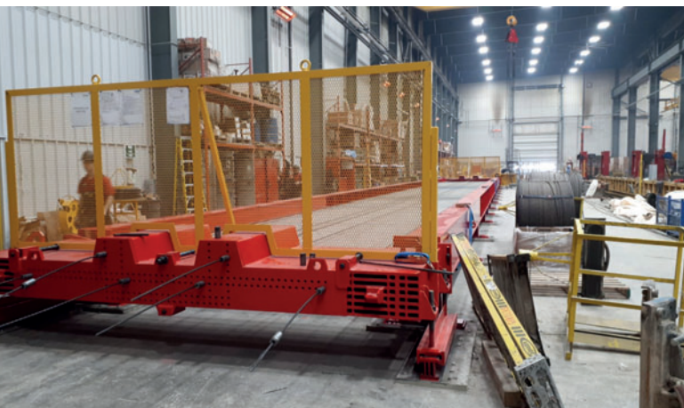
2.7m x 34m self-stressing universal casting bed with 560 tons of prestressing capacity
