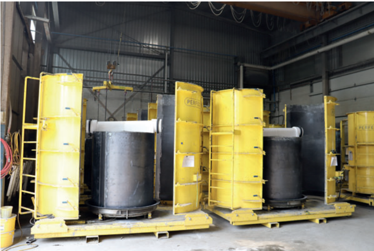
The moulds have a two-piece mould shell and can be pulled apart symmetrically.
