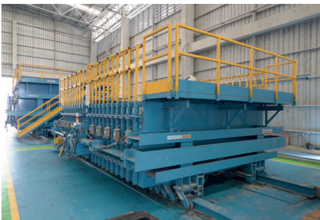
With the new battery moulds, Sansiri produces partition walls and fencing walls.
