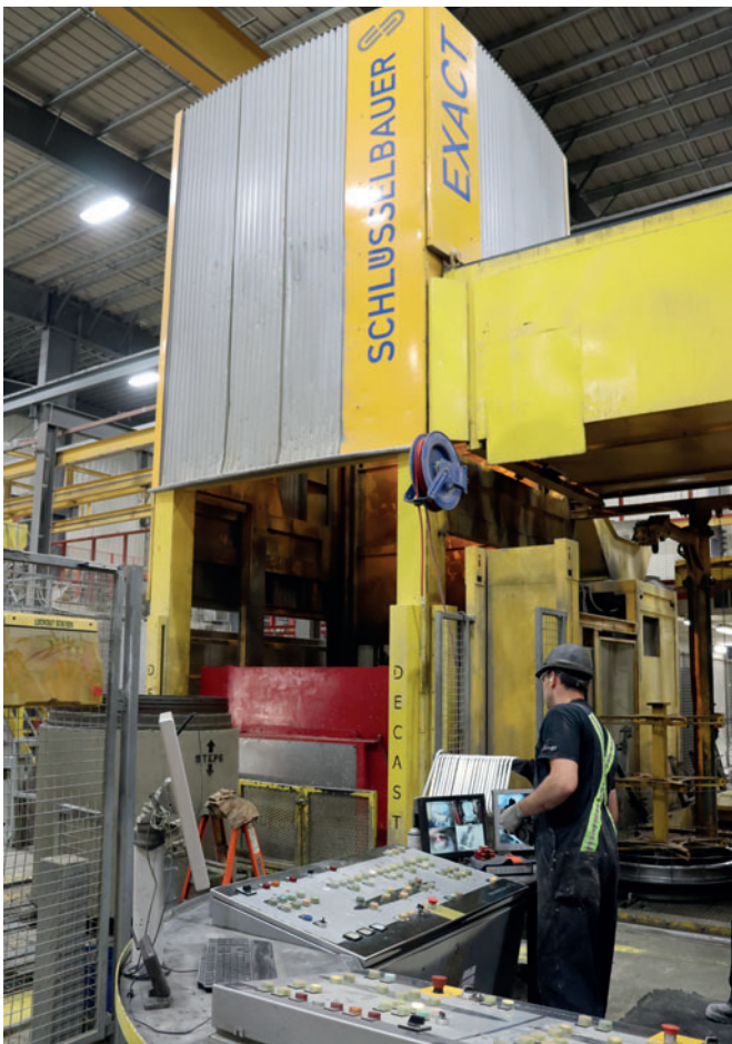
Also successful in continuous operation: Schlüssellbauer Exact pipe and manhole component machine
