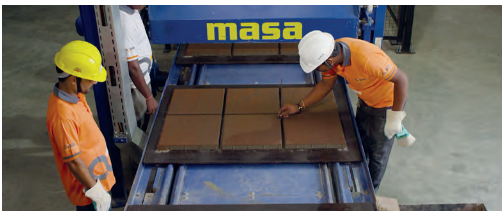
Manual quality control of the freshly produced concrete slabs
