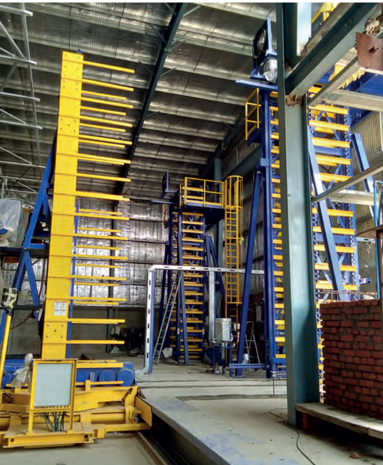
Assembly of elevator, lowerator and finger car
