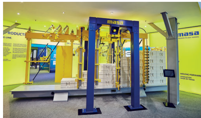
Side cutting and profiling station for AAC products
